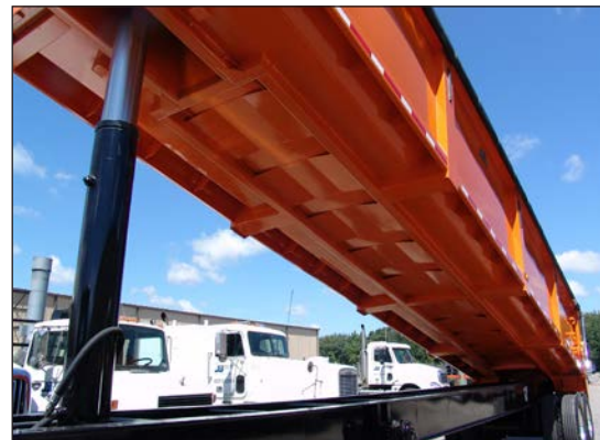
Lighter weight high hard steel cushioned floor plates absorb impact while maintaining the integrity of the trailer.
