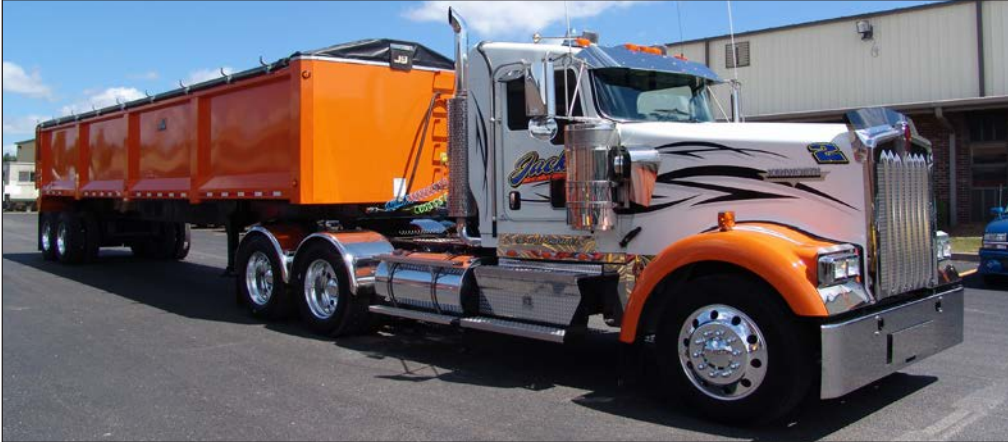
The body design is a constant taper from front to rear, which allows the material to slide out easier, eliminating load hang-ups while discharging the payload.
