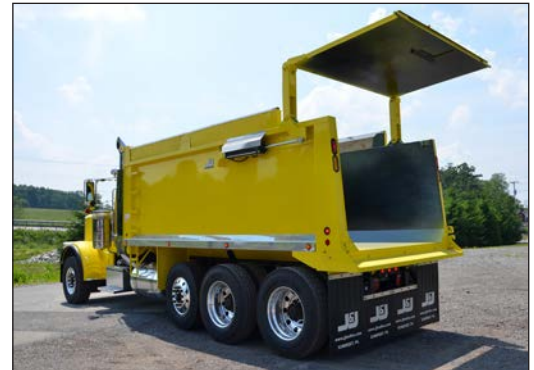
The hydraulic lift tailgate option prevents tailgate damage from large objects and functions as a conventional tailgate for standard aggregate hauling.
