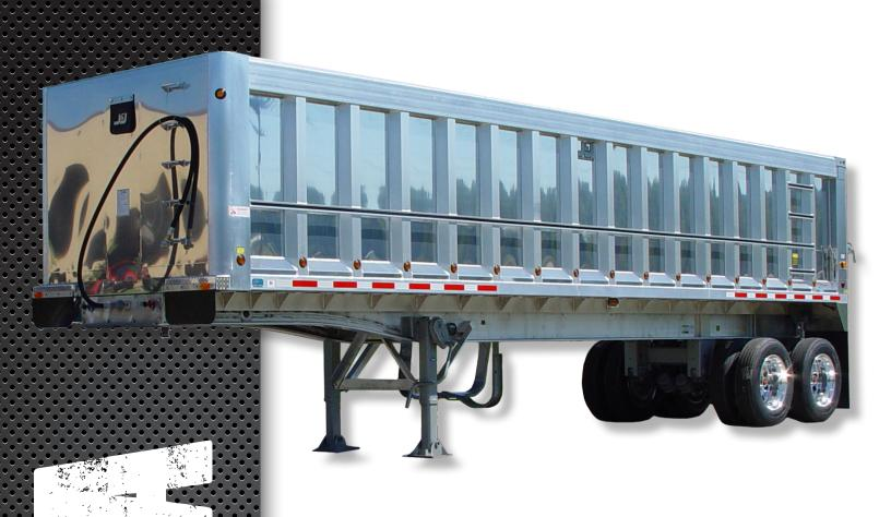
Aluminum body, steel frame dump trailers are engineered for excavation and construction material hauling.
