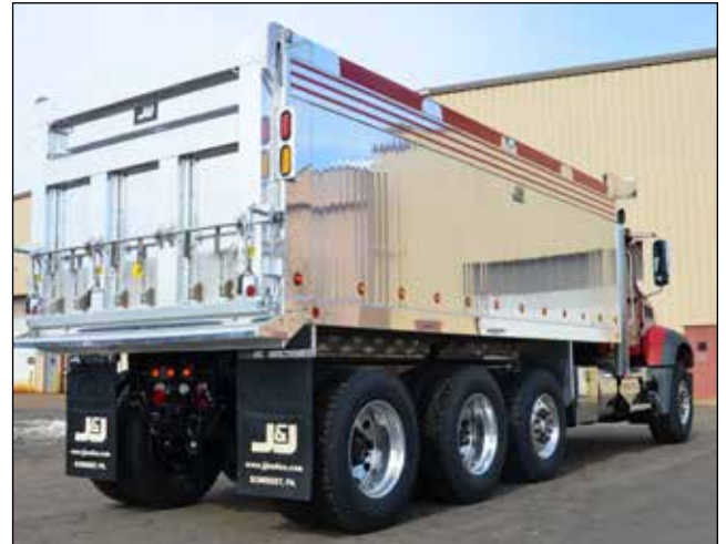
Polished aluminum is one of the most popular options on J&J EVO bodies.
