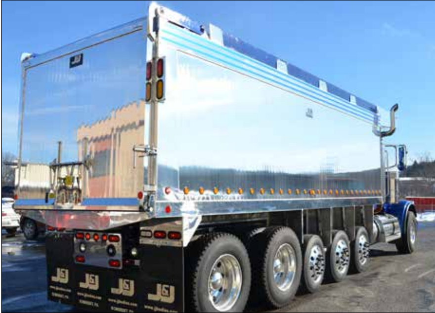
The reinforced double wall side panels create excellent insulating properties for asphalt haulers.
