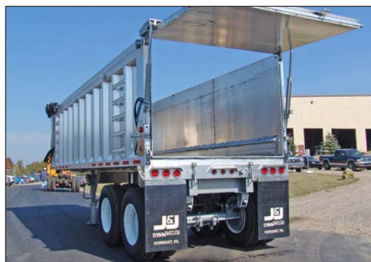
Trailer shown with optional hydraulic tailgate and full rubber seal.
