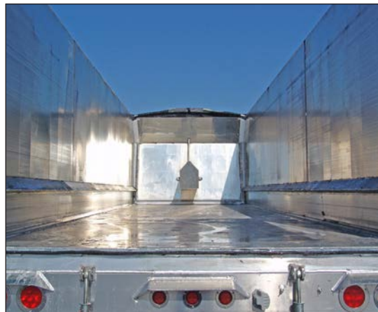
Ejector ram cylinder sized to completely unload trailer. Replaceable UHMW wipers on sides and bottom.
