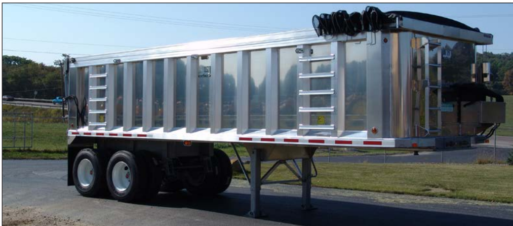
Trailer shown with optional bulkhead ladder (Man door standard). Ejector controls mounted on driver's side bulkhead.
